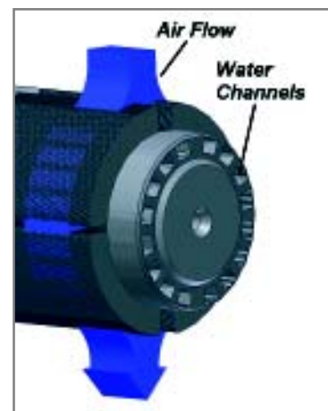
Air flow over the core.
